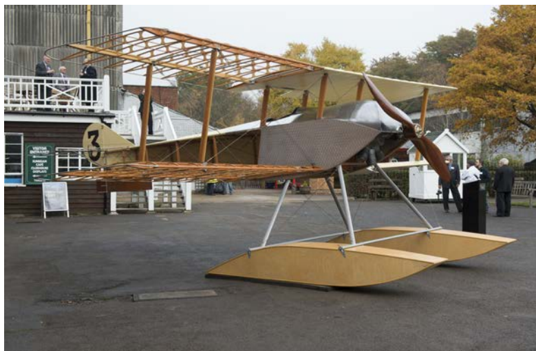
Floatplane showing uncovered structure
