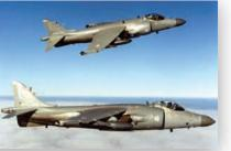
The 1988 British Aerospace Sea Harrier FA2 was developed from Falklands War experience. Improvements included a new radar, larger fuel tanks and long range air-to-air missiles
