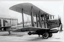
The Sopwith T1 Cuckoo torpedo bomber, just too late for the war, was retained post-war as the only RAF torpedo aeroplane which could operate from aircraft carriers
