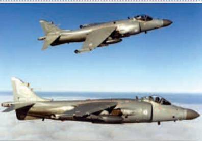
**The 1988 British Aerospace Sea Harrier FA2 was developed from Falklands War experience. Improvements included a new radar, larger fuel tanks and long range air-to-air missiles**
