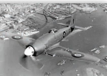
**The 1945 Hawker Sea Fury with a top speed of 465 mph was the pinnacle of the piston engined fighter and the last built by Hawker**
