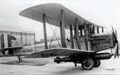
**The Sopwith TI Cuckoo torpedo bomber, just too late for the war, was retained post-war as the only RAF torpedo aeroplane which could operate from aircraft carriers**
